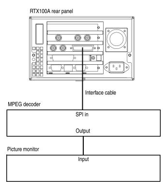
Figure 1-5: Equipment connection for the functional check
