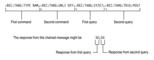
Figure 3-31: Example of chaining commands and queries
