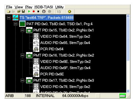
Figure 2-11: Hierarchy view of the transport stream file
