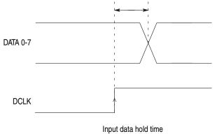
Figure A-1: Timing diagram of the DVB-SPI interface
